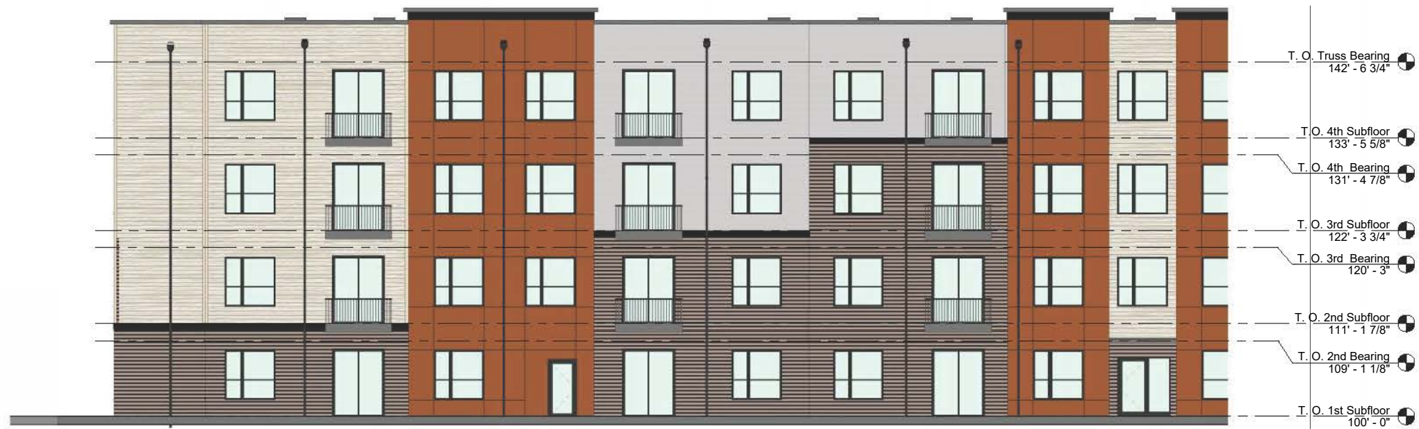
1 BUILDING A - REAR ELEVATION AREA 2 1/8" = 1'-0"
