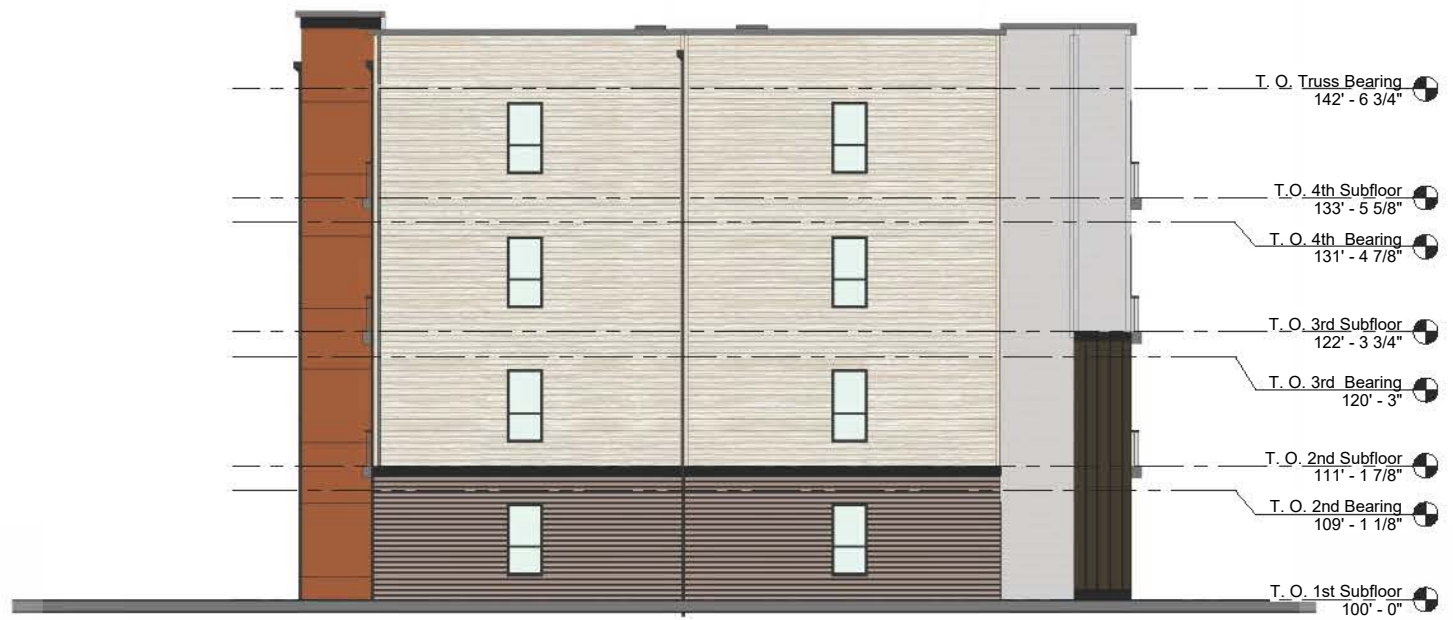
2 BUILDING A - LEFT ELEVATION - AREA 1 1/8" = 1'-0" 0 4' 8' 16'
