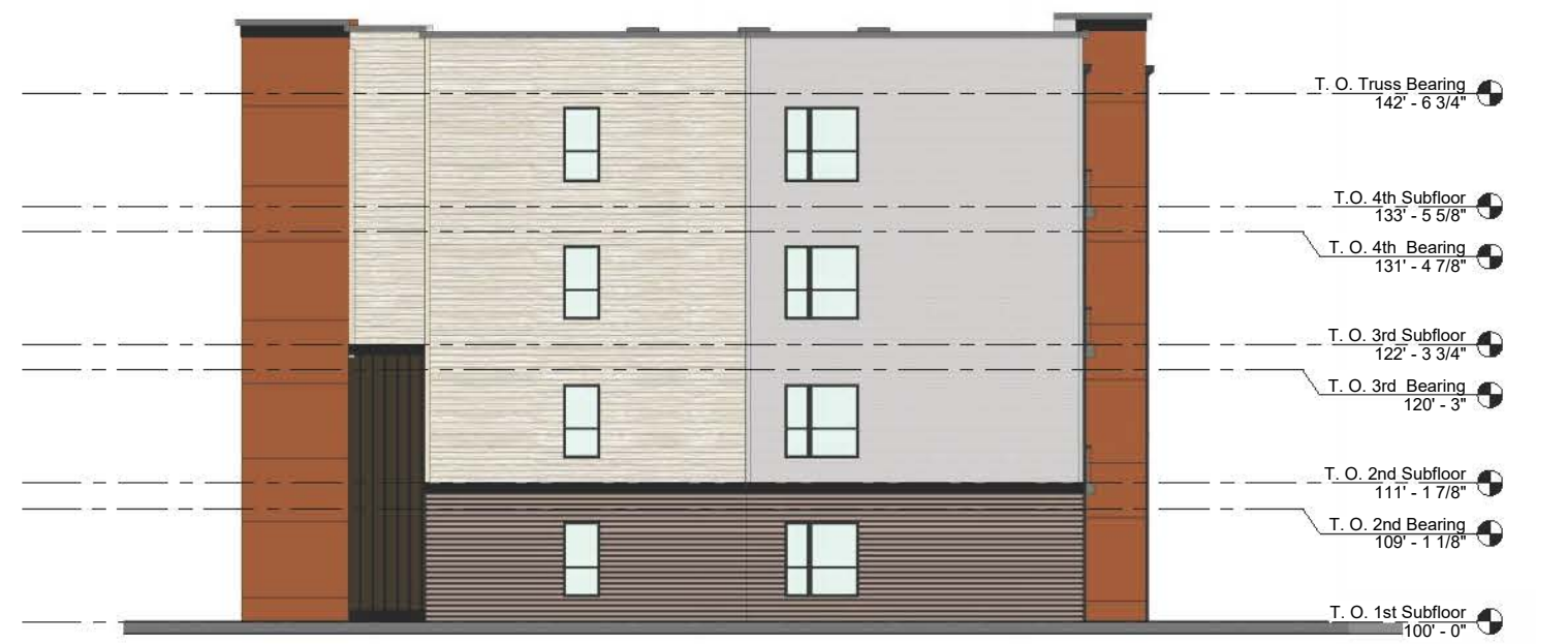
1 BUILDING B - LEFT ELEVATION - AREA 1 1/8" = 1'-0" 0 4' 8' 16'
