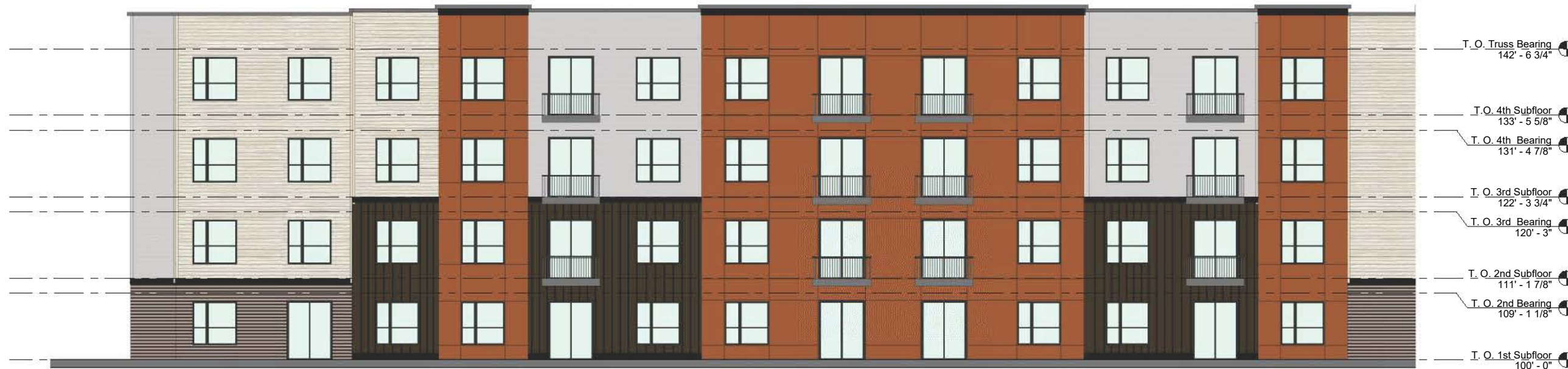
2 BUILDING B - REAR ELEVATION - AREA 2 1/8" = 1'-0"
