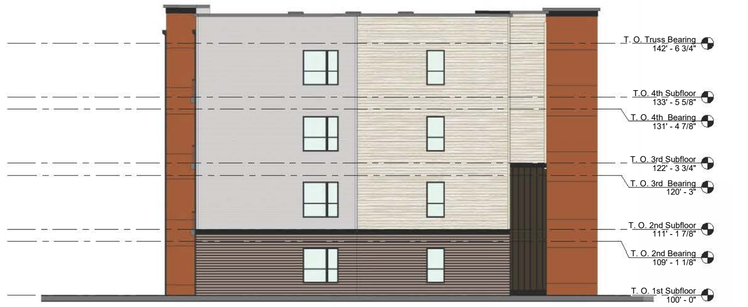
2 BUILDING B - RIGHT ELEVATION - AREA 2 1/8" = 1'-0" 0 4' 8' 16'
