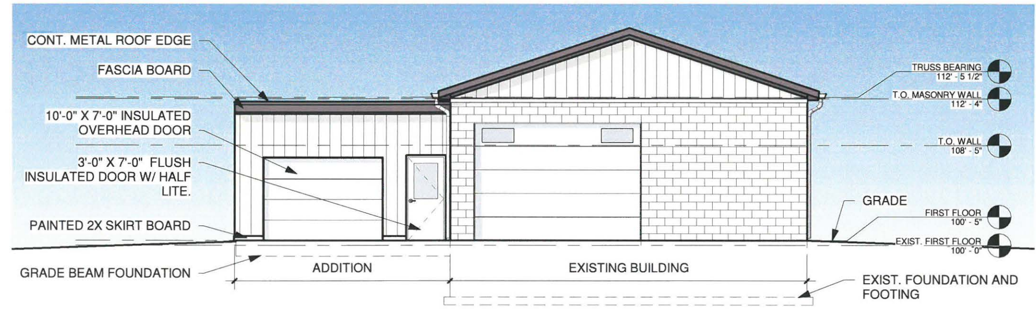
2 EXTERIOR ELEVATION - EAST ELEVATION 1/8" = 1'-0"
