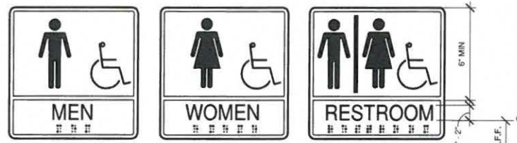
4 ADA TOILET ROOM SIGNS 3" = 1'-0" PLAQUE WITH VISUAL, TACTILE & BRAILLE CHARACTERS, PICTOGRAM, AND SYMBOL OF ACCESSIBILITY INSTALLED ON THE WALL ADJACENT TO THE LATCH SIDE OF THE DOOR. SIGNS SHALL HAVE WHITE SYMBOLS, CHARACTERS, AND LETTERS ON BLACK BACKGROUND. VERIFY EXACT LANGUAGE WITH OWNER. WHERE THERE IS NO WALL SPACE ON THE LATCH SIDE OF A SINGLE DOOR, SIGNS SHALL BE ON THE NEAREST ADJACENT WALL. SIGNS CONTAINING TACTILE CHARACTERS SHALL BE LOCATED SO THAT A CLEAR FLOOR AREA 18 INCHES MINIMUM BY 18 INCHES MINIMUM, CENTERED ON THE TACTILE CHARACTERS, IS PROVIDED BEYOND THE ARC OF ANY DOOR SWING BETWEEN THE CLOSED POSITION AND 45 DEGREE OPEN POSITION. SIGNS WITH TACTILE CHARACTERS SHALL BE PERMITTED ON THE PUSH SIDE OF DOORS WITH CLOSERS AND WITHOUT HOLD-OPEN DEVICES.
