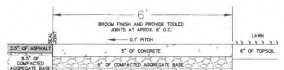
CONCRETE SIDEWALK TYPE B
