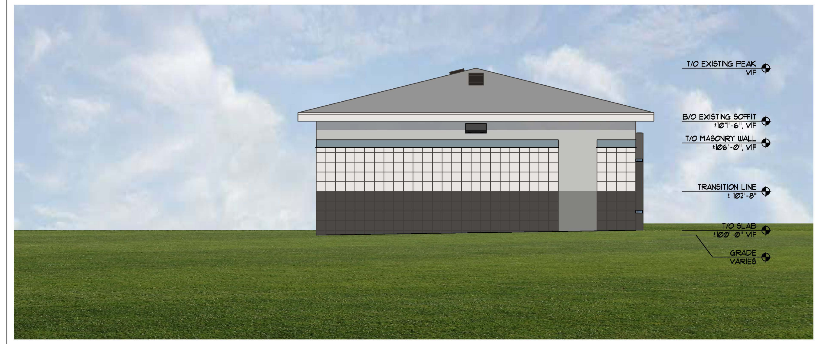
EXTERIOR ELEVATION - OUTBUILDING SOUTH FACE SCALE: 1/4" = 1'-0" 4
