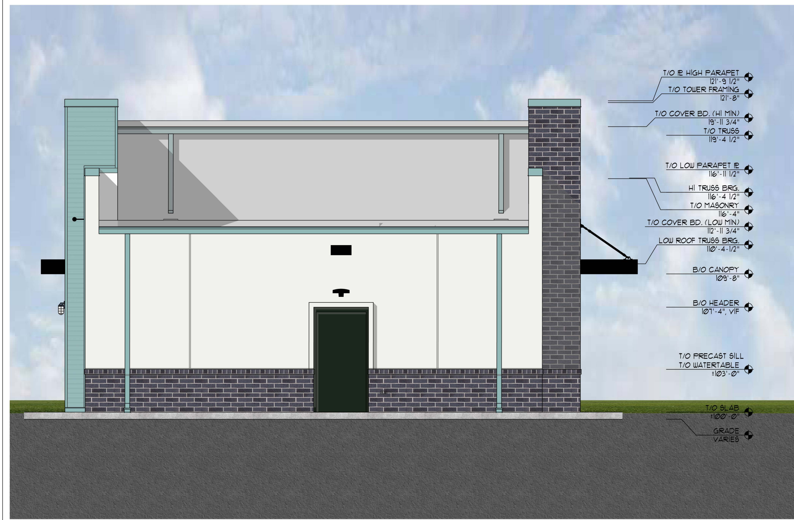
EXTERIOR ELEVATION - WEST FACE
