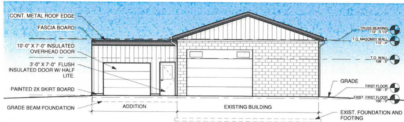
② EXTERIOR ELEVATION - EAST ELEVATION 1/8" = 1'-0"
