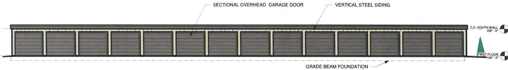
2 FLOOR PLAN - SOUTH ELEVATION 3/32" = 1'-0"
