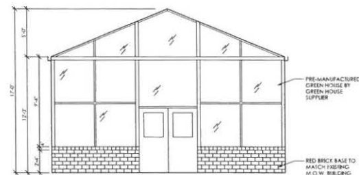
EAST GREENHOUSE ELEVATION SCALE: 1/4"=1'-0"
