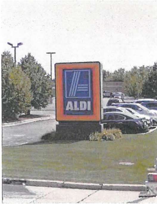
C RETRO-FIT EXISTING MONUMENT w/ L.E.D. Scale: NTS - INSTALL NEW WHITE L.E.D. LIGHTING INTO EXISTING 8'-¾" x 9'-6½" MONUMENT SIGN
