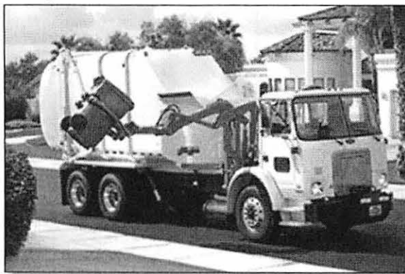
Figure 4 Example of Automated Side Load Trucks
