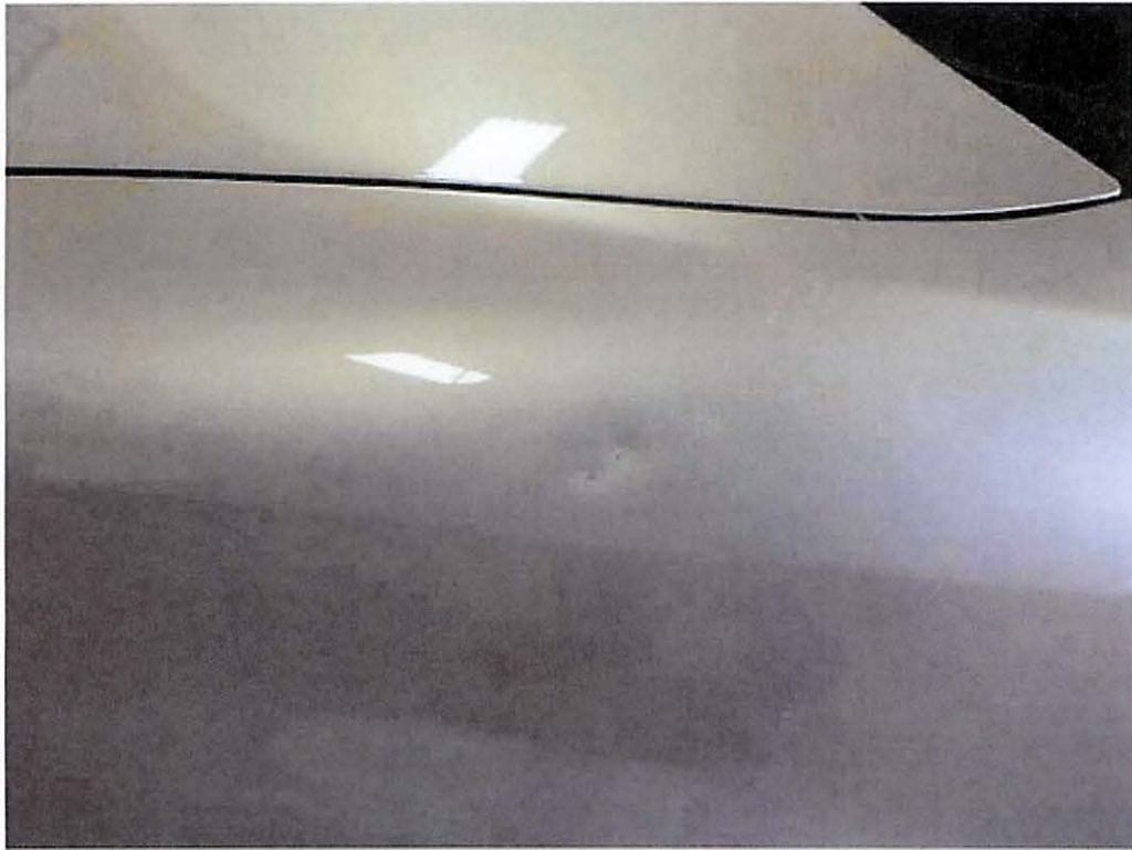
LF FENDER DAMAGE
