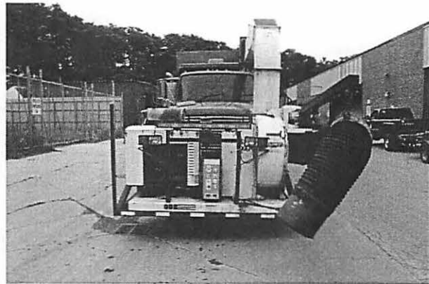
Image 4 – View of the front of the leaf collector in its mounted position on the vehicle.
