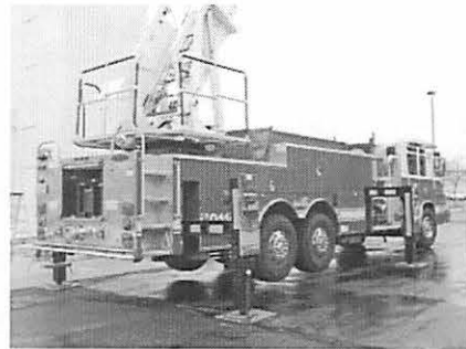
FIRE DEPARTMENT LADDER UNDERGOES ANNUAL TESTING TO ASSURE PROPER OPERATION AND SAFETY.
