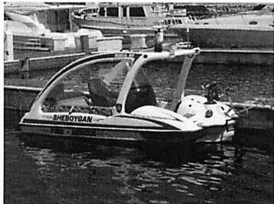
THE SHEBOYGAN FIRE BOAT SERVES AS A SEARCH AND RESCUE PLATFORM AND ALSO HAS WATER BASED FIREFIGHTING CAPABILITY WITH A 750 GPM PUMP AND MASTER STREAM NOZZLE.
