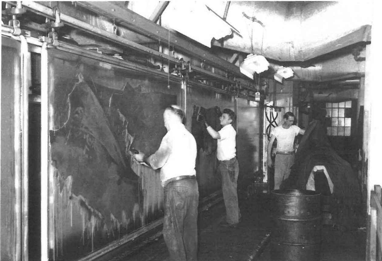
Figure 9: Interior of main tanning sections (Sections 7 and 8), scraping hides, 1957
