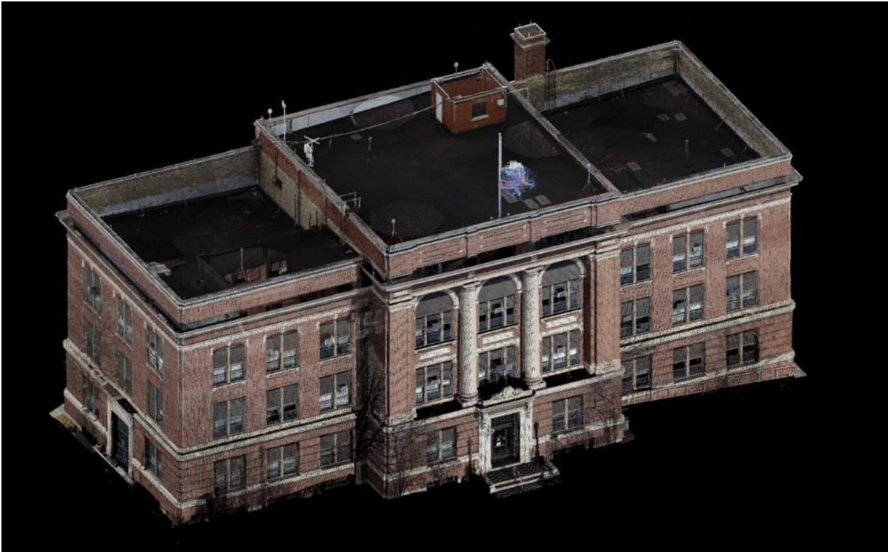
Figure 3: Sheboygan City Hall colorized 3D laser scan image.
