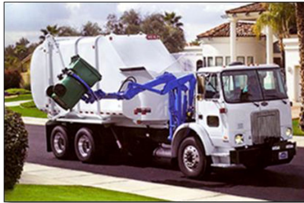
Figure 4 Example of Automated Side Load Trucks
