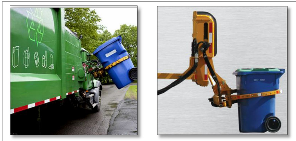
Figure 5 Example of Automated Side Load Lifting Arms
