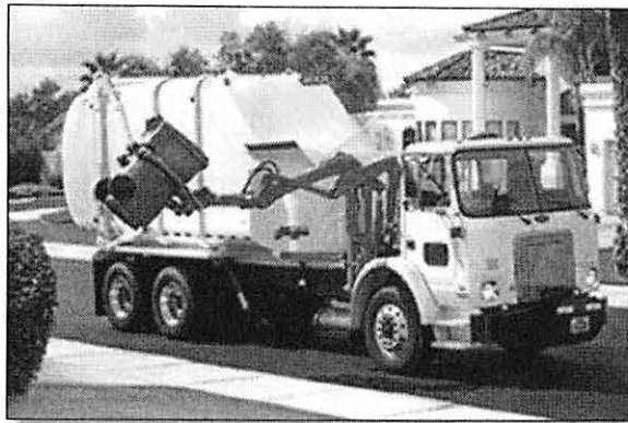
Figure 4 Example of Automated Side Load Trucks
