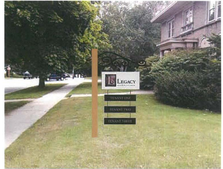
Cedar post approximately 8' tall and extend out approximately 4'. Signs hanging center with stand. Sandblasted signs with steel painted posts attaching it to cedar post (4x4)
